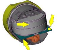
The three yellow arrows on the TN4 electronics indicate the contacts of the WN.LN.I.
